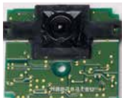
▲ Example in which a photosensor and an optical component are combined (optics module)
