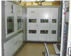
Thin-film crystal growth with MOCVD equipment
